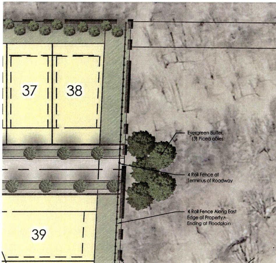
NORTHEAST ROADWAY BUFFER ENLARGEMENT 1"=40'-0"
