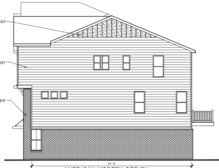
AMERICAN MODERN DESIGN RIGHT SIDE ELEVATION 28% MASONRY
