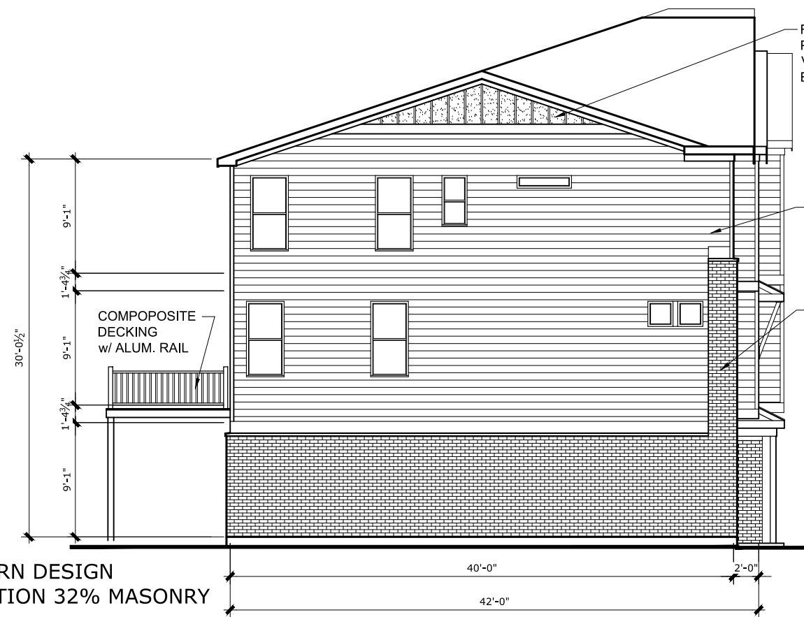
AMERICAN MODERN DESIGN REAR ELEVATION 6-UNIT BUILDING REAR ELEVATION 30% MASONRY
