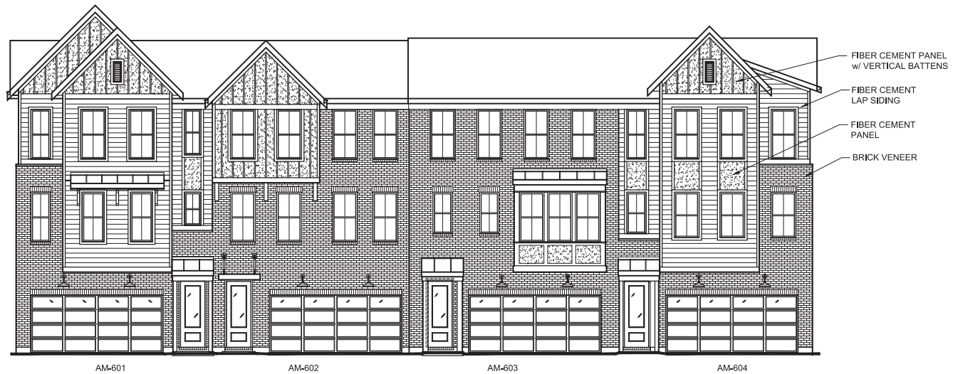
BROOKLINE FRONT ELEVATION AMERICAN MODERN EXTERIOR DESIGN 4-HOME BUILDING FRONT ELEVATION 55% MASONRY
