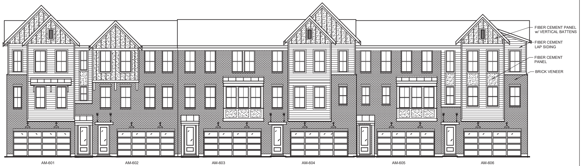
BROOKLINE FRONT ELEVATION AMERICAN MODERN EXTERIOR DESIGN 6-HOME BUILDING FRONT ELEVATION 58% MASONRY
