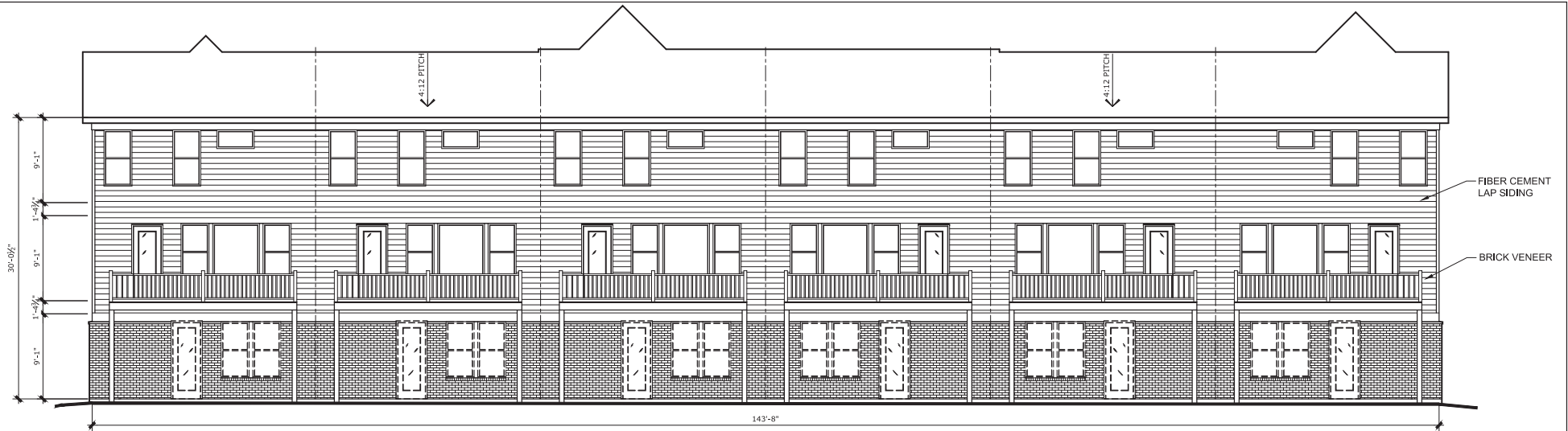
AMERICAN MODERN DESIGN REAR ELEVATION 6-UNIT BUILDING REAR ELEVATION 30% MASONRY
