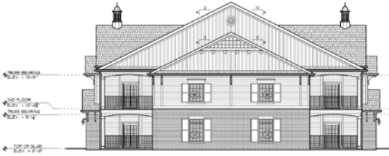
2 BUILDING TYPE V - SIDE EXTERIOR ELEVATION SCALE 1/8" = 1'-0"
