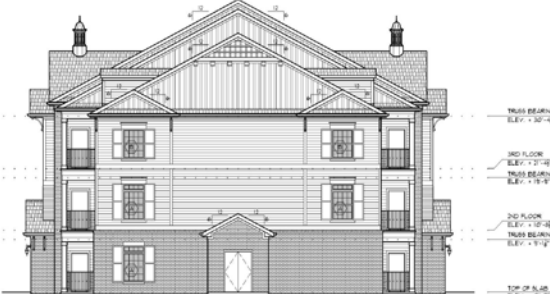
1 BUILDING TYPE II - SIDE EXTERIOR ELEVATION SCALE 1/8" = 1'-0"
