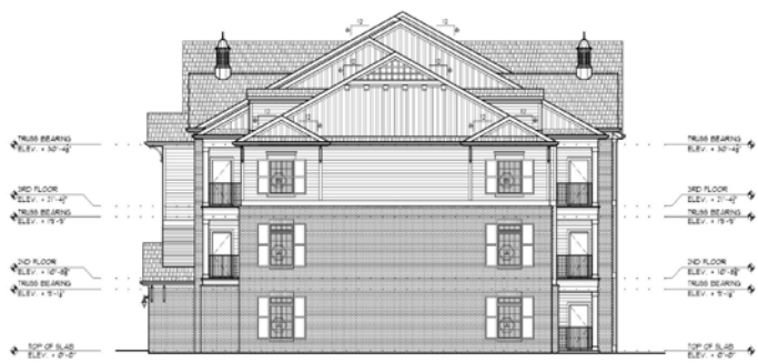
2 BUILDING TYPE I - SIDE EXTERIOR ELEVATION SCALE: 1/8" = 1'-0"
