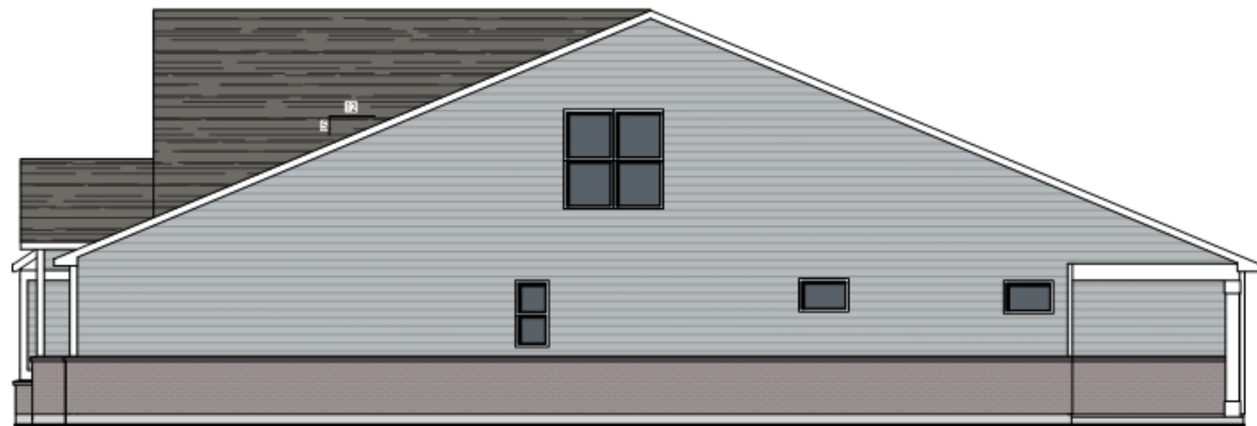
Side Elevation Brick Water Table
