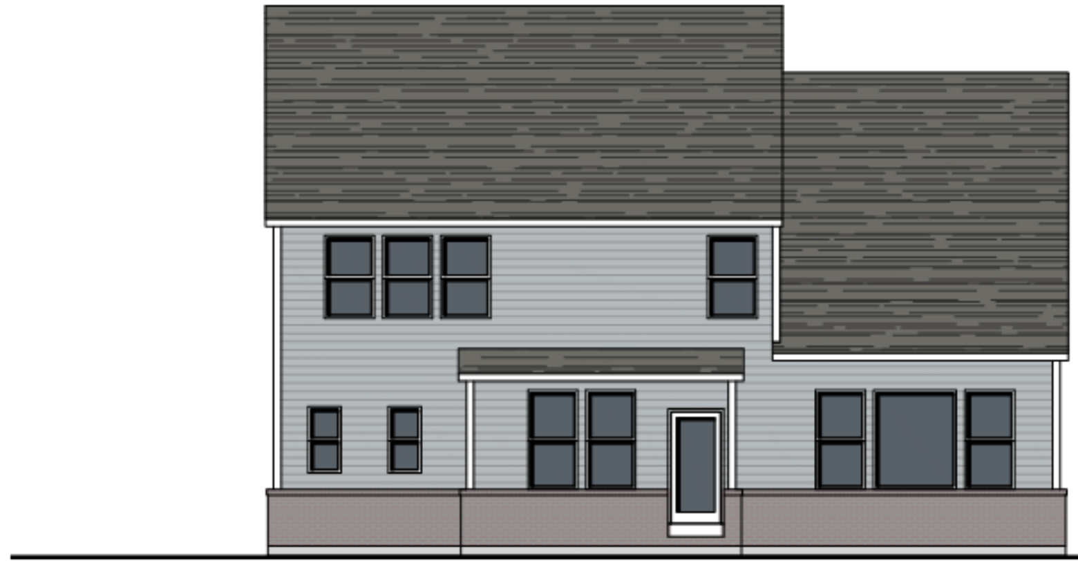
Rear Elevation Brick Water Table & Sunroom
