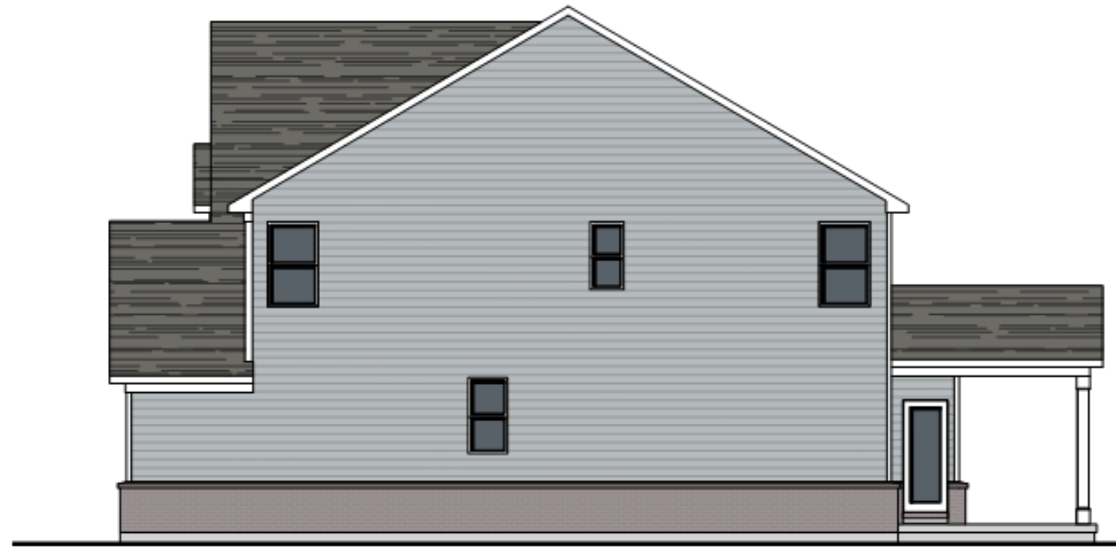
Side Elevation Brick Water Table
