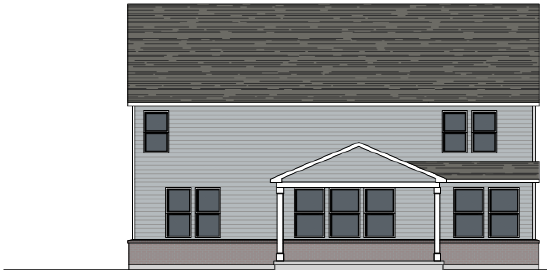
Rear Elevation Brick Water Table
