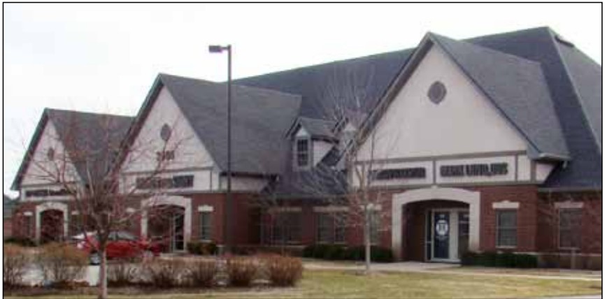
FIGURE 5.3(8): PITCHED ROOF - ROOF LINE MODULATION
