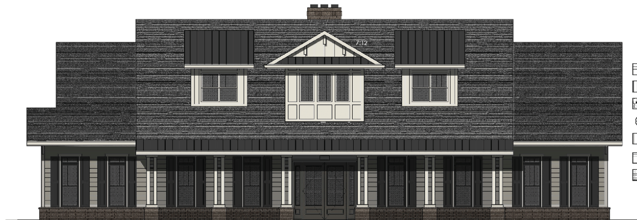
1 BUILDING #6 FRONT ELEVATION (AS VIEWED FROM PARKING LOT) SCALE: 1/8"=1'-0" BUILDING HEIGHT: 27'-8 1/2" (MEASURED TO RIDGE)
