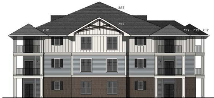
2 BUILDING #1 SIDE ELEVATION (AS VIEWED FROM NORTHEAST) SCALE: 1/8"=1'-0" (MIXED BEDROOM UNIT BUILDING - L-SHAPED) (24 UNITS)
