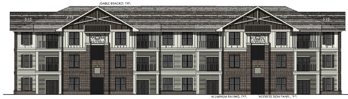
BUILDING #14 FRONT / REAR ELEVATIONS SCALE: 1/8"=1'-0" BUILDING HEIGHT: 35'-1 1/4"
