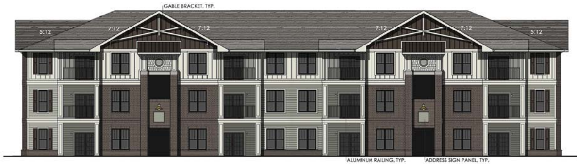
BUILDING #14 FRONT / REAR ELEVATIONS SCALE: 1/8"=1'-0" BUILDING HEIGHT: 35'-1 3/4"
