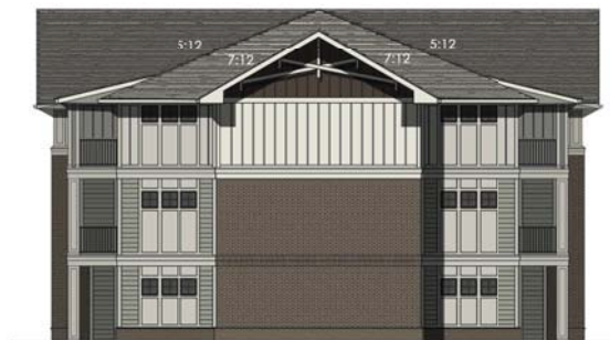
BUILDING #14 SIDE ELEVATIONS SCALE: 1/8"=1'-0"
