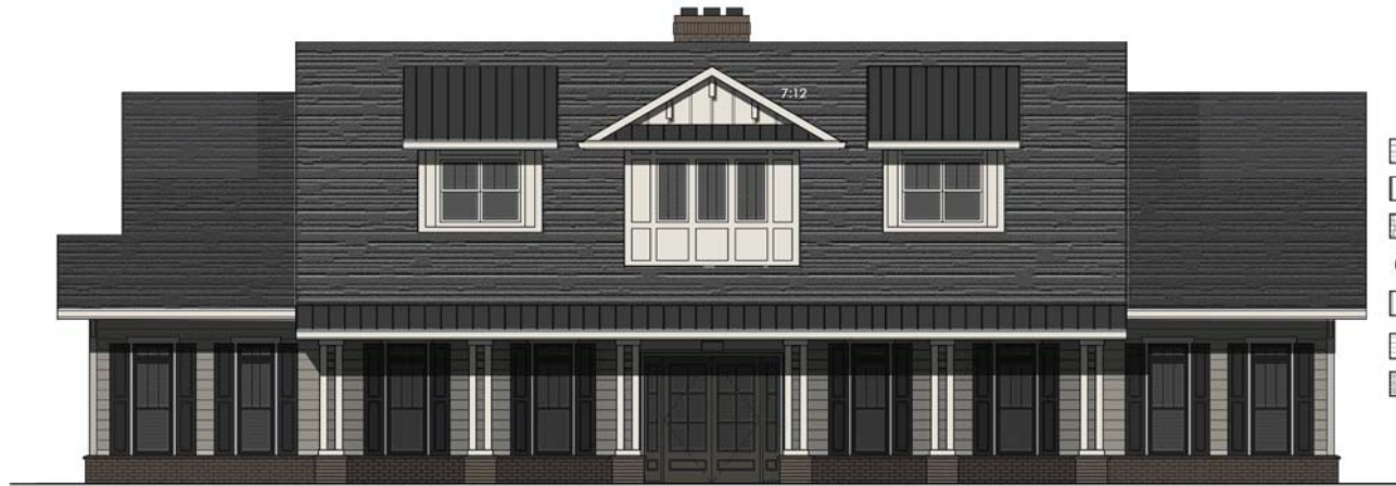
BUILDING #6 FRONT ELEVATION (AS VIEWED FROM PARKING LOT) SCALE: 1/8"=1'-0" BUILDING HEIGHT: 27'-8 3/4" (MEASURED TO RIDGE)
