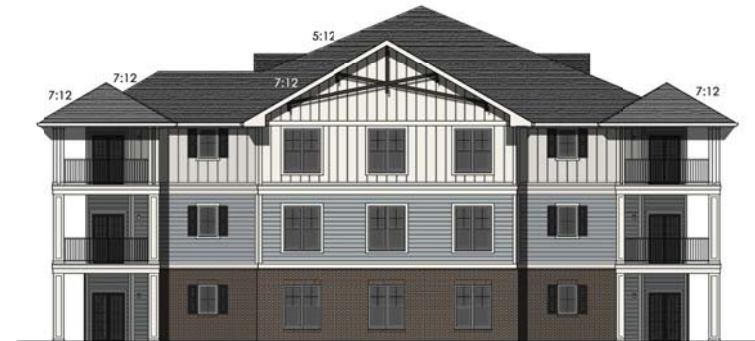
3 BUILDING #5 SIDE ELEVATION (SOUTH) SCALE: 1/8"=1'-0"
