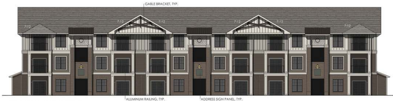
1 BUILDING #16 FRONT ELEVATION SCALE: 1/8"=1'-0" BUILDING HEIGHT: 37'-7 1/4"
