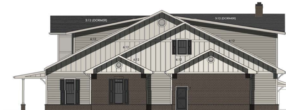
2 BUILDING #6 SIDE ELEVATION (NORTH) SCALE: 1/8"=1'-0"
