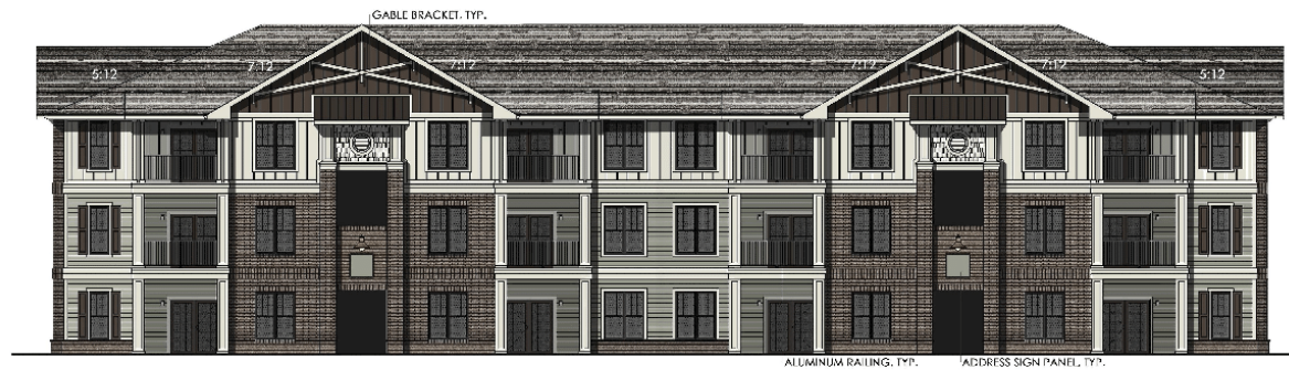
BUILDING #14 FRONT / REAR ELEVATIONS SCALE: 1/8"=1'-0" BUILDING HEIGHT: 35'-1 1/4"
