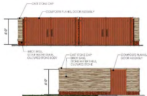
TRASH ENCLOSURE ELEVATIONS
