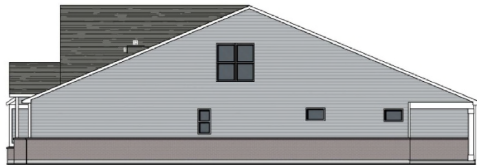
Side Elevation Brick Water Table
