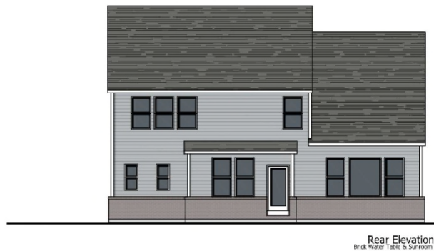
Rear Elevation Brick Water Table & Sunroom
