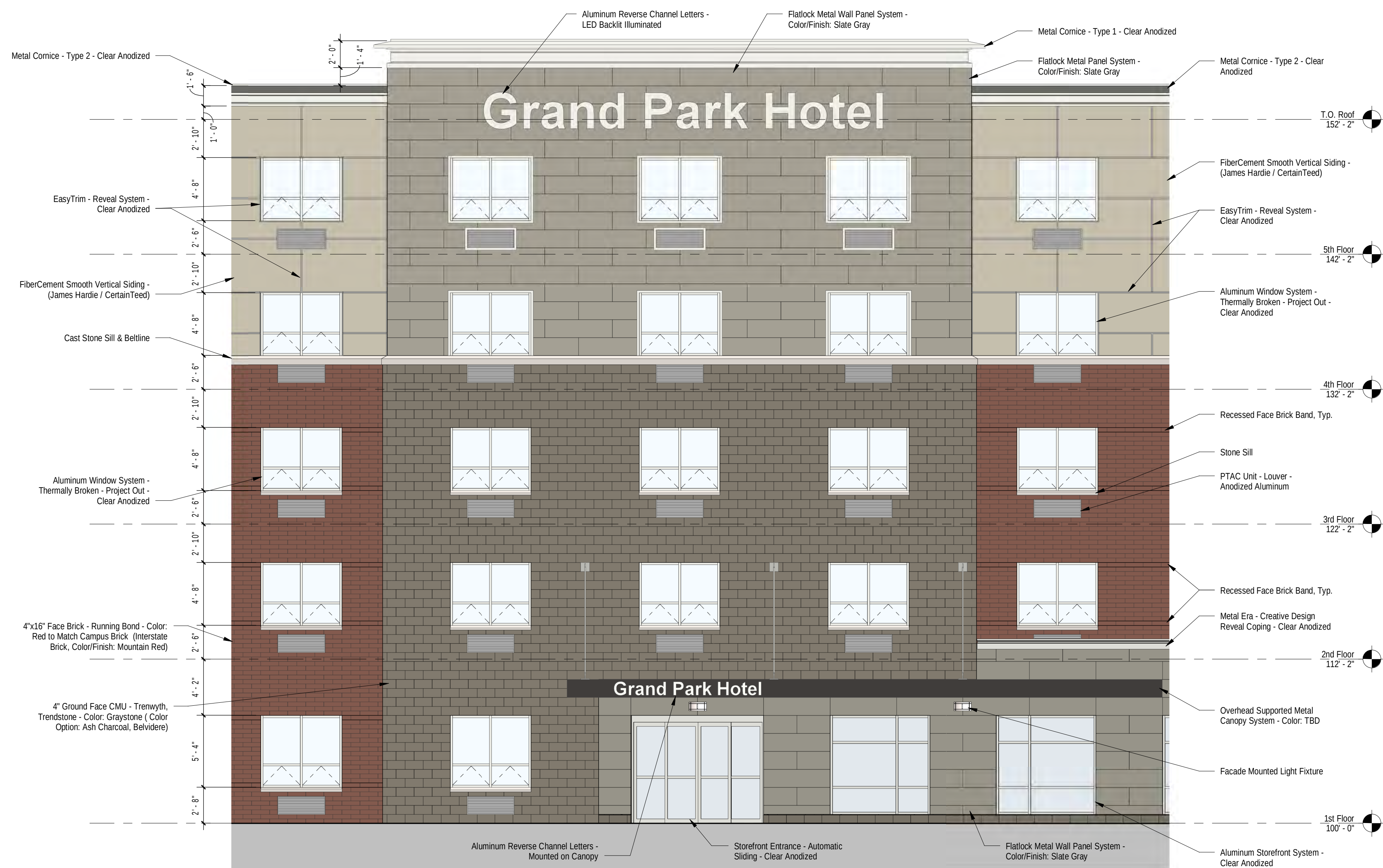
5 Enlarged West Elevation - Entrance
