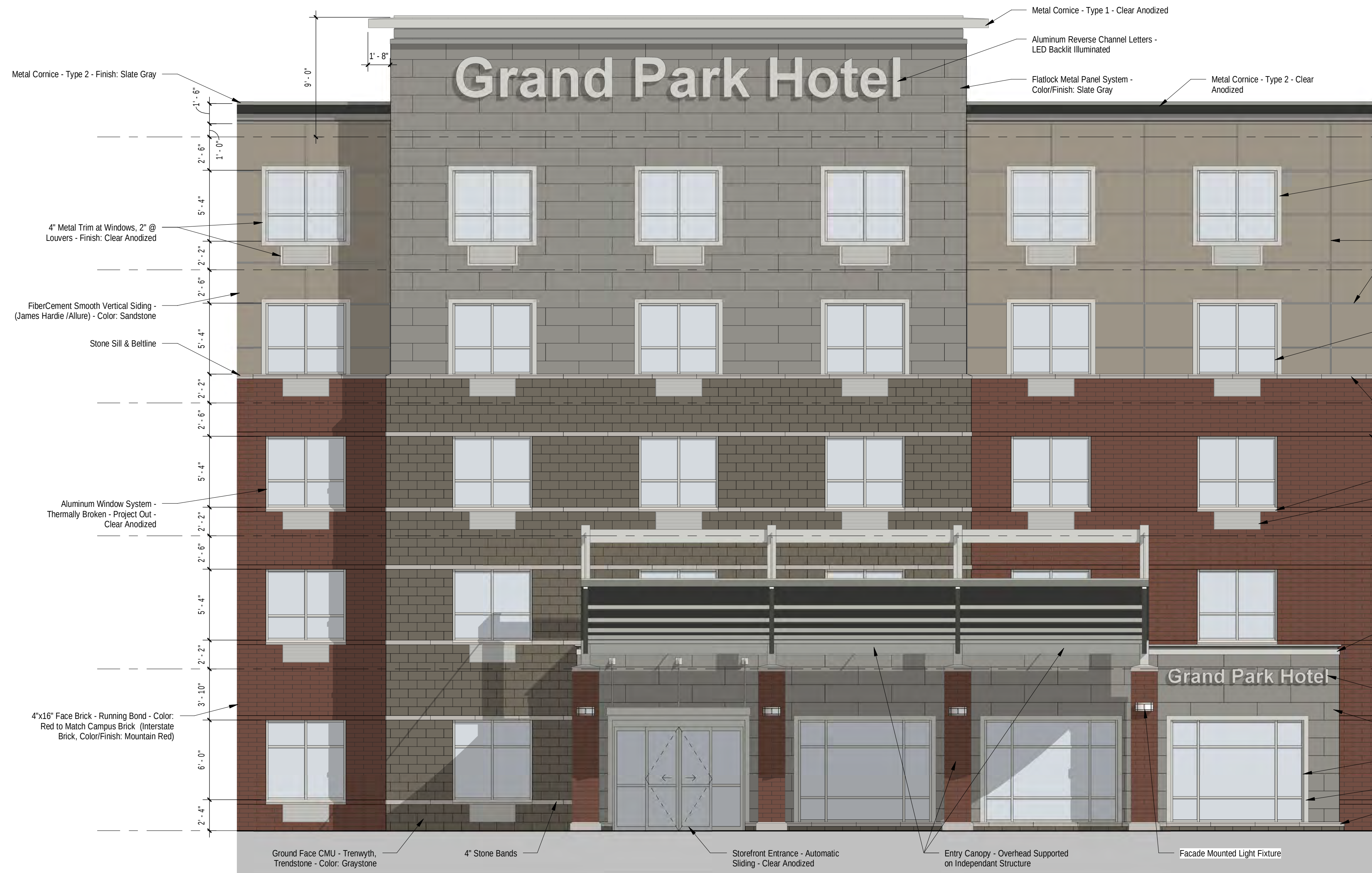
5 Enlarged West Elevation - Entrance
