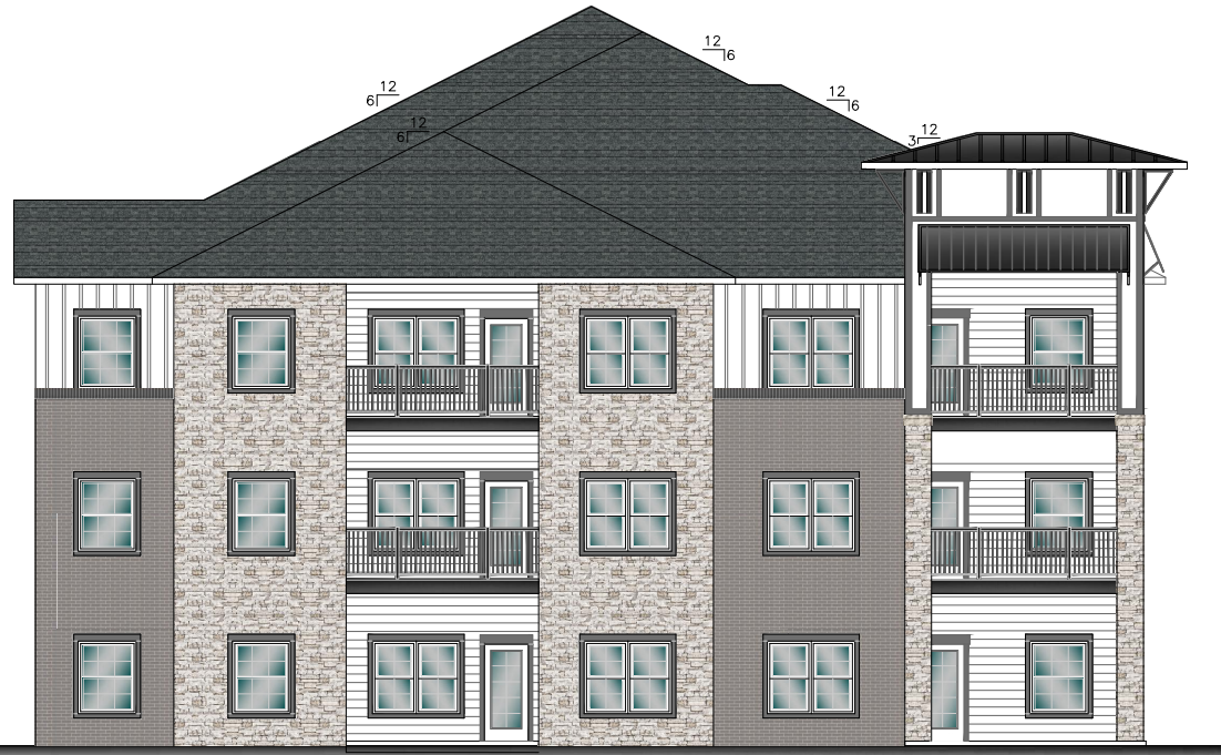
D 3 STORY - SIDE ELEVATION A0 NOT TO SCALE
