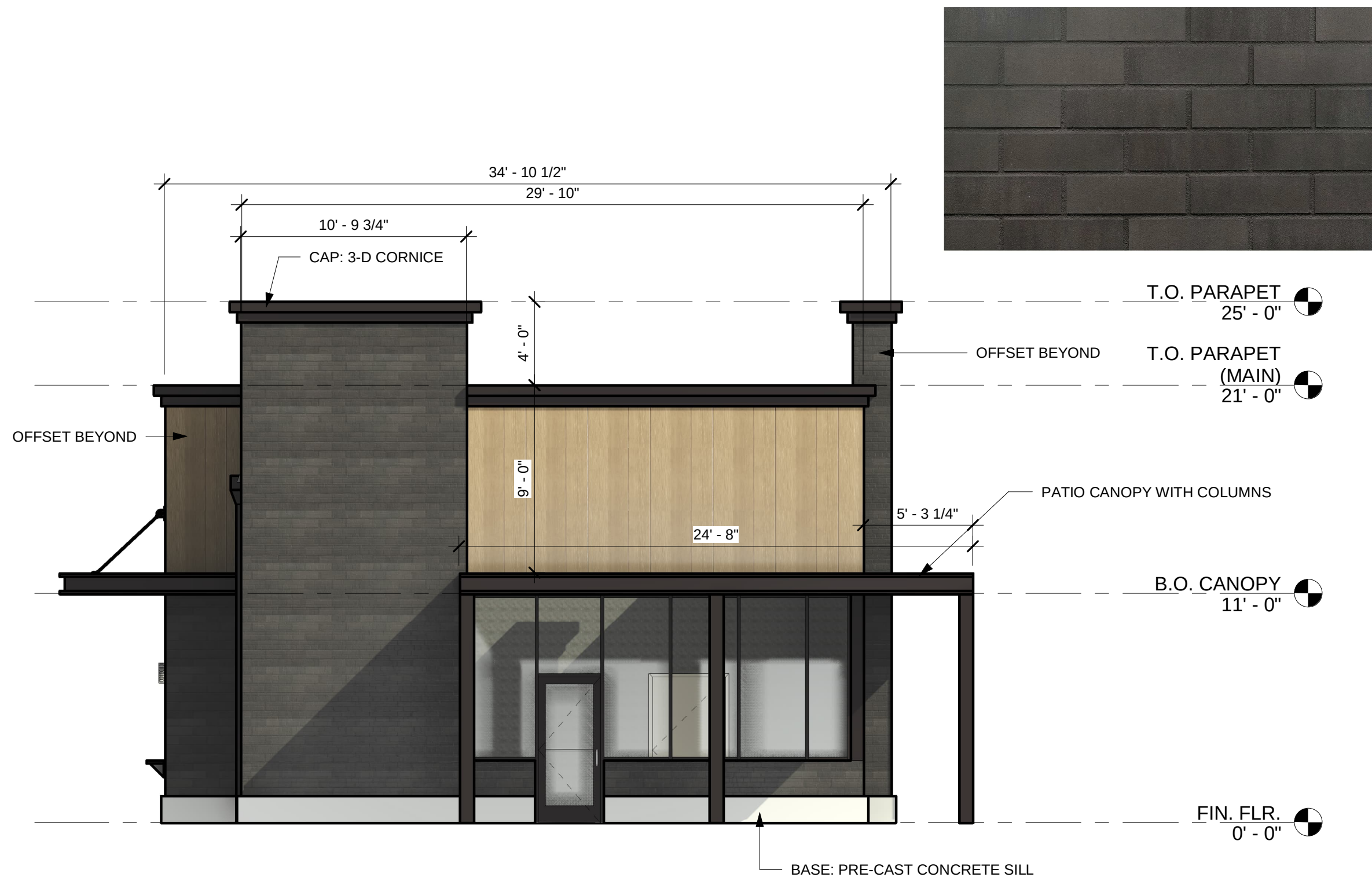
SOUTH ELEVATION PRELIM
