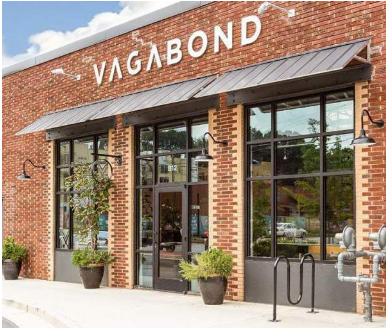
2" x 4-1/2" ALUM. STOREFRONT- BASIS OF DESIGN: MFR: TUBELITE SERIES: T14000 COLOR: BLACK ANODIZED
