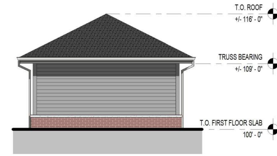
8 9-BAY GARAGE - LEFT SIDE ELEVATION 1/8" = 1'-0"
