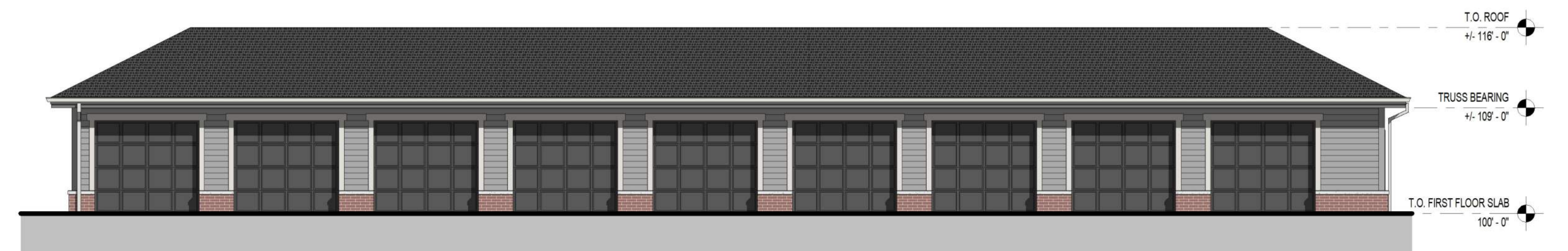
3 9-BAY GARAGE - FRONT ELEVATION 1/8" = 1'-0"
