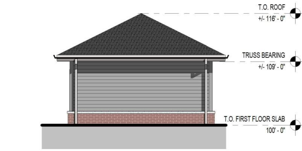
9 8-BAY GARAGE - SIDE ELEVATION 1/8" = 1'-0"
