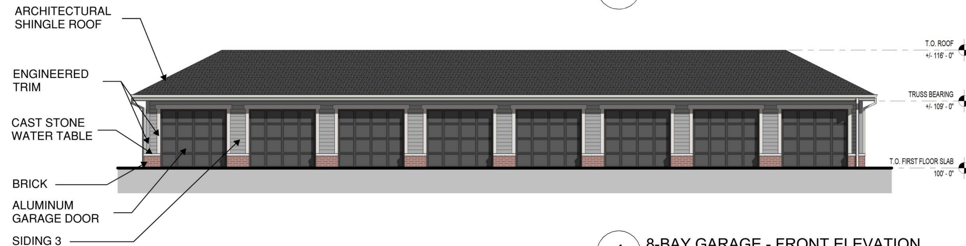
4 8-BAY GARAGE - FRONT ELEVATION 1/8" = 1'-0"
