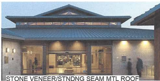
STONE VENEER/STNDNG SEAM MTL ROOF
