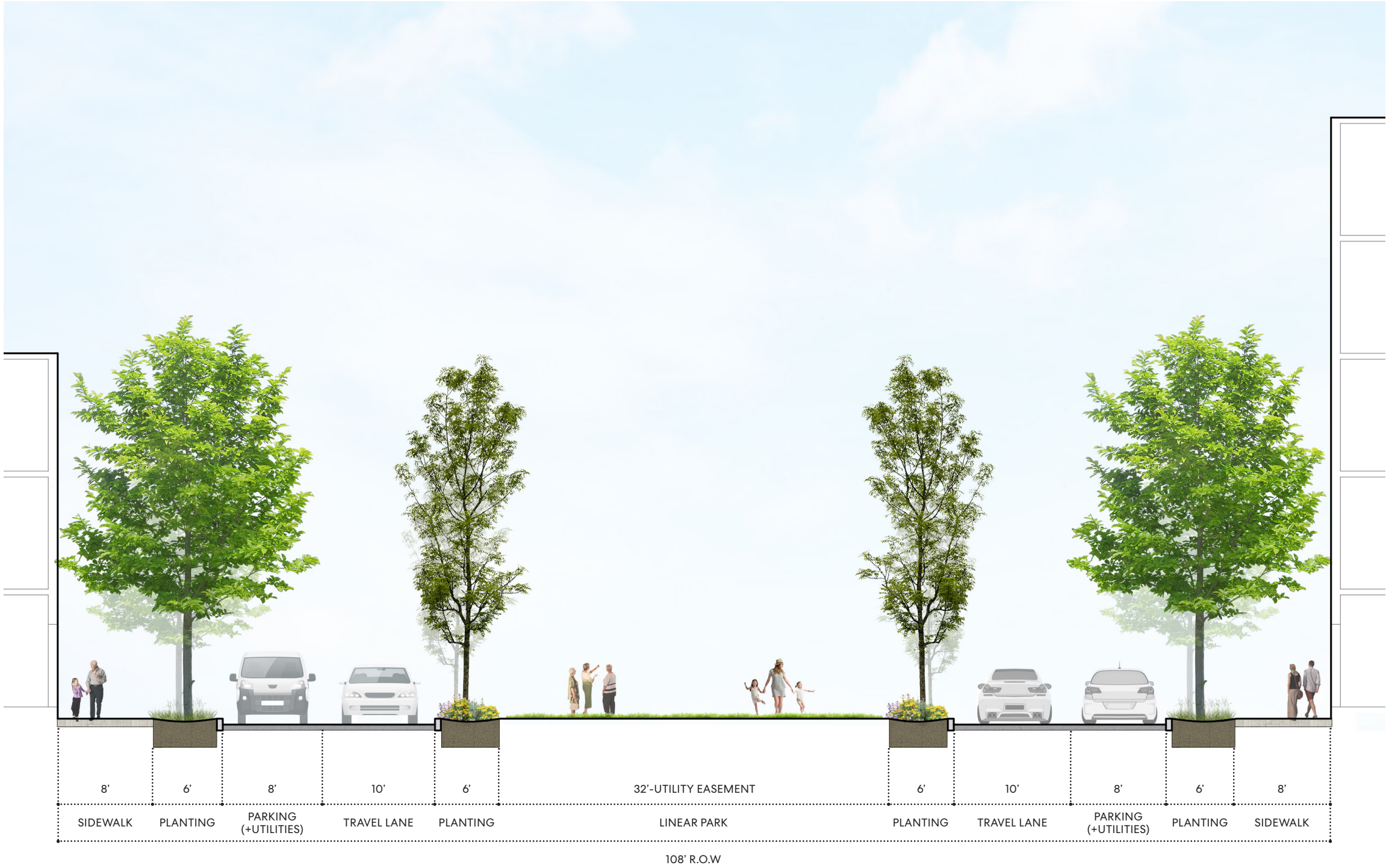
Section 11: North Area Utility Easement - Boulevard Condition
