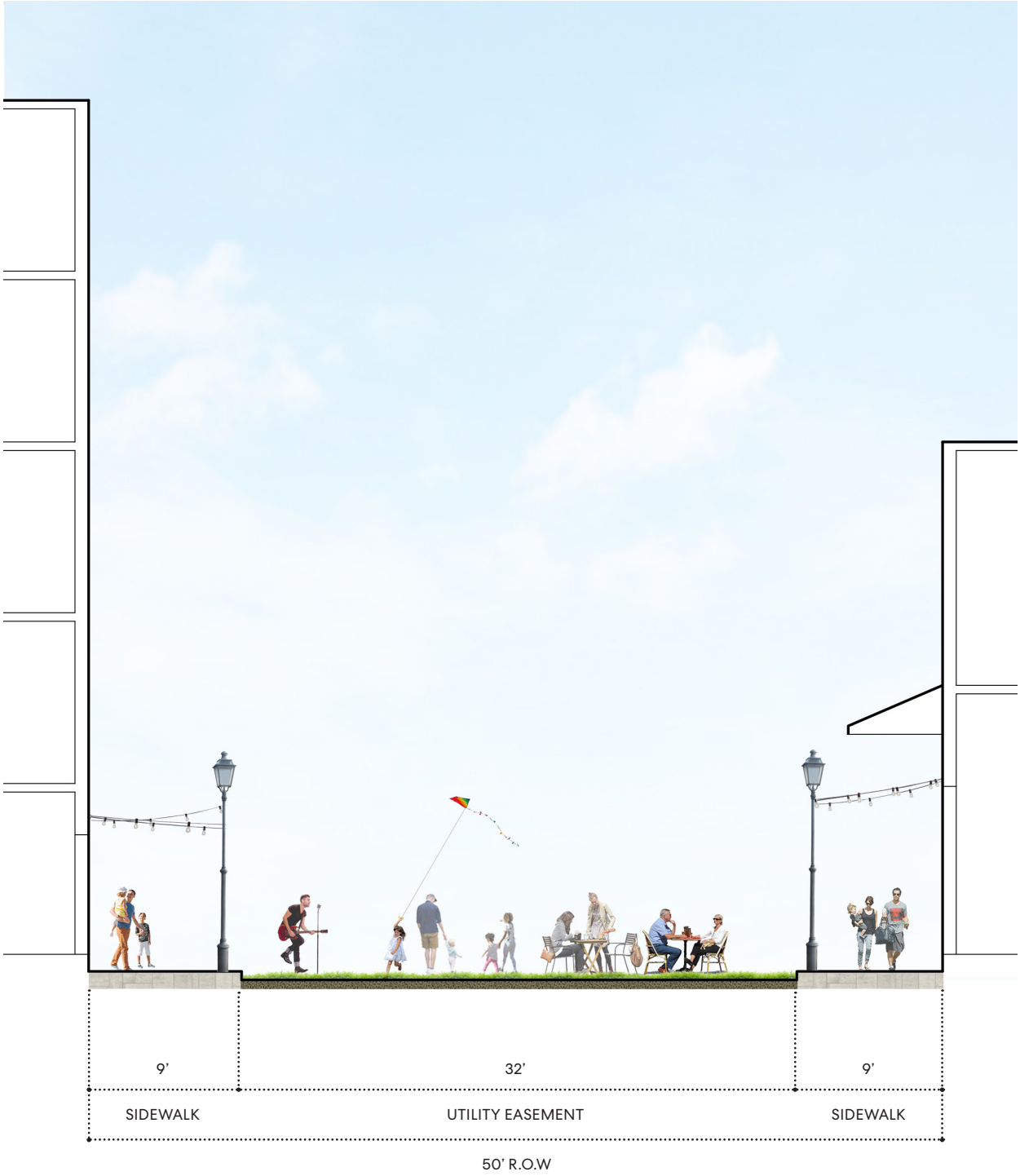
Section 10: North Area Utility Easement - Paseo Condition
