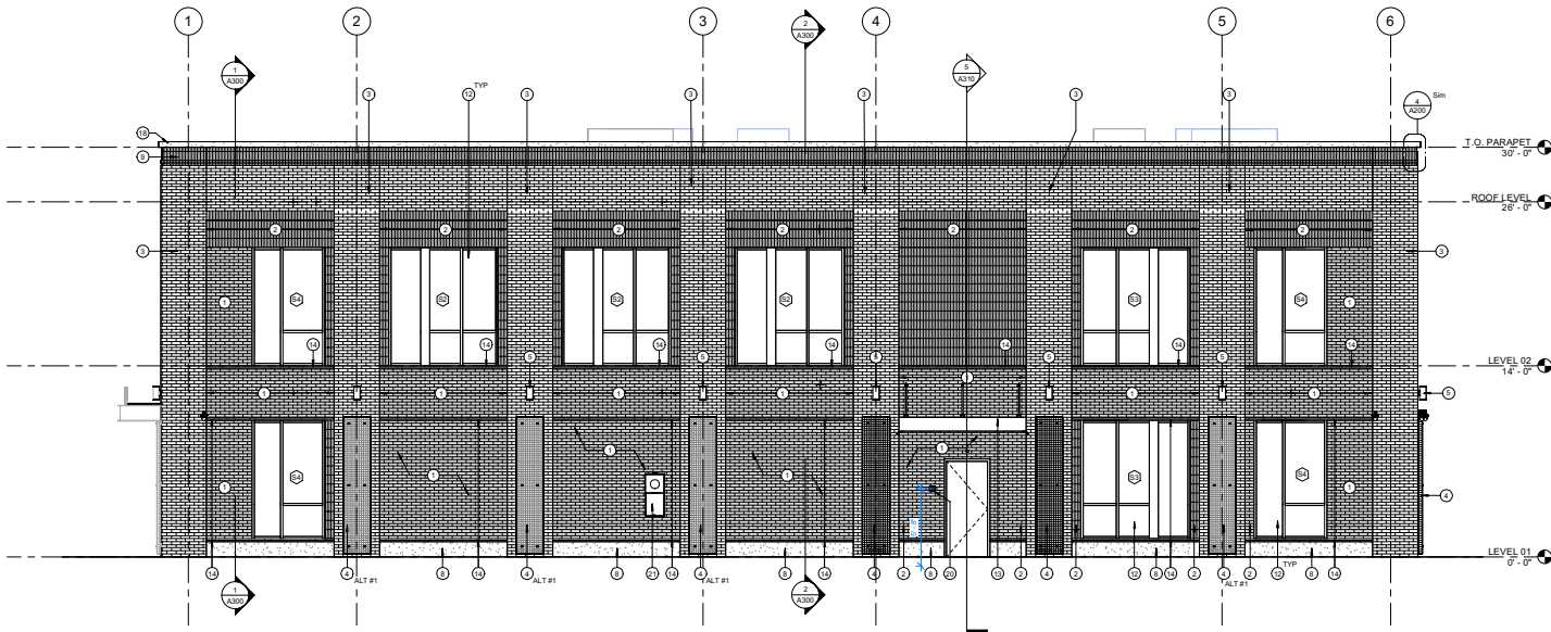
2 SOUTH EXTERIOR BUILDING ELEVATION 1/4" = 1'-0"
