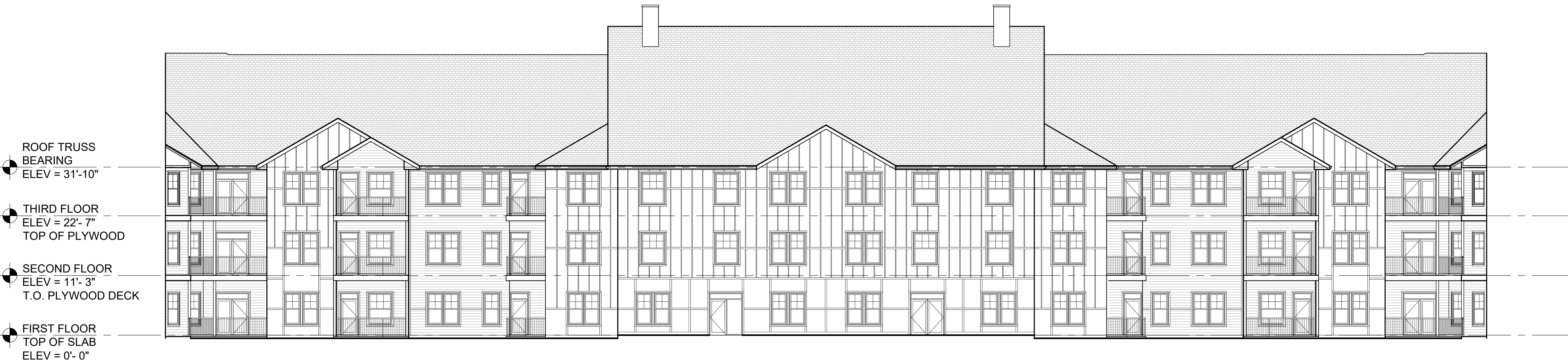
7 BUILDING A - WEST COURTYARD EXTERIOR ELEVATION SCALE: 3/32" = 1'-0"
