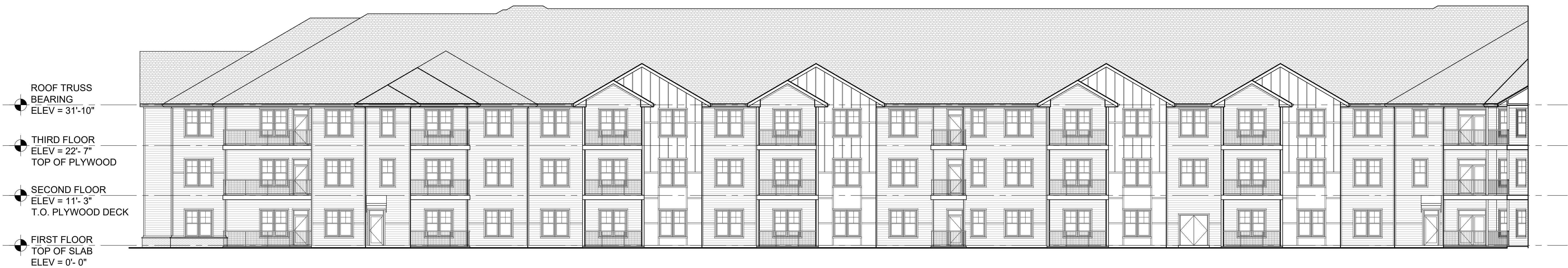
5 BUILDING A - SOUTH COURTYARD EXTERIOR ELEVATION SCALE: 3/32" = 1'-0"
