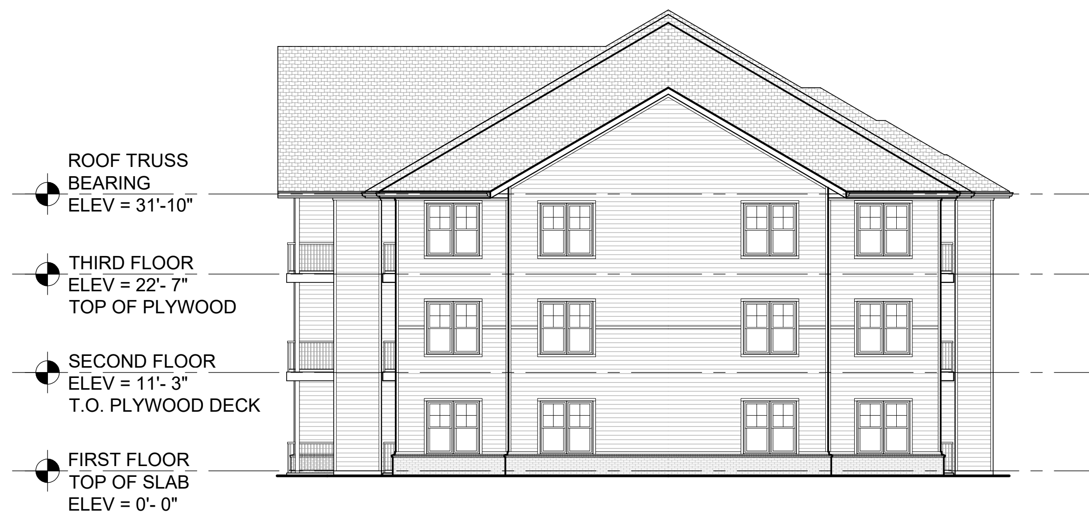
4 BUILDING A - WEST EXTERIOR ELEVATION SCALE: 3/32" = 1'-0"
