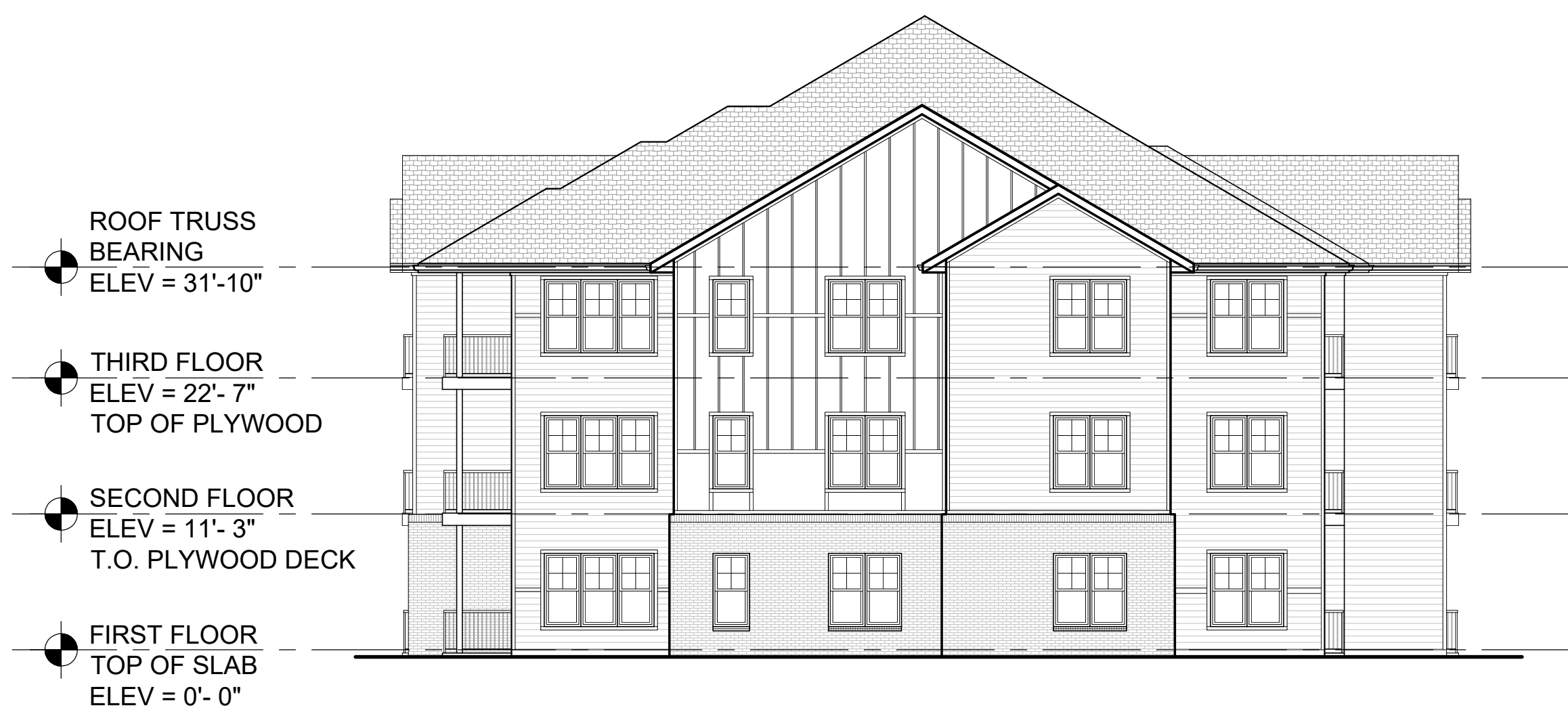
2 BUILDING B - SOUTH EXTERIOR ELEVATION - NORTH REVERSED SCALE: 3/32" = 1'-0"
