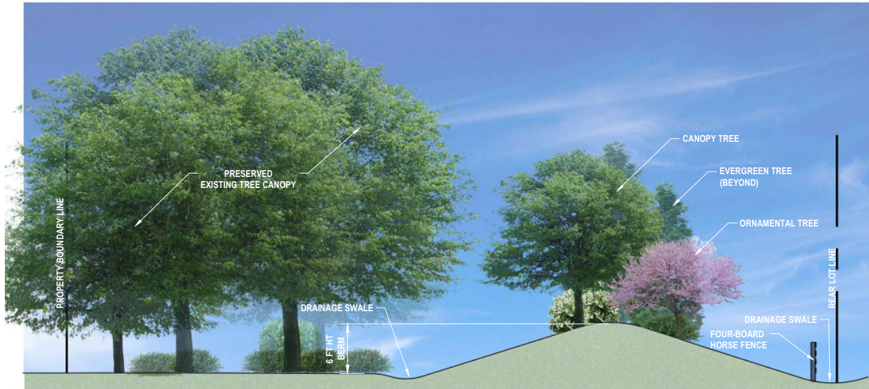
BUFFER YARD - CROSS SECTION A-A
