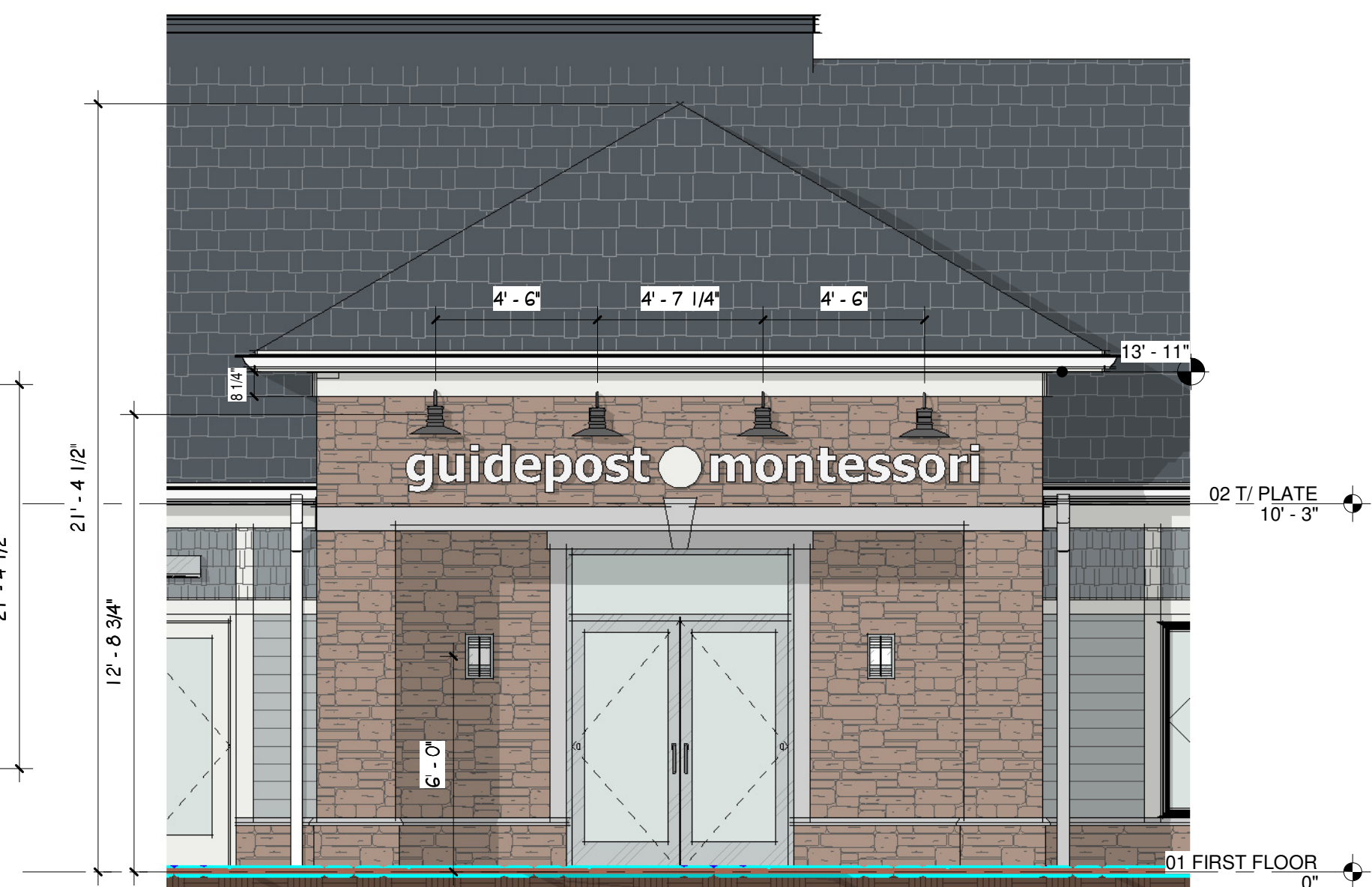
5 WEST ENTRY ELEVATION 1/4" = 1'-0"
