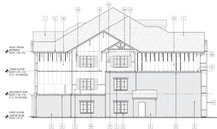
4 SIDE ELEVATION W/ RISER ROOM SCALE: 1/8" = 1'-0"
