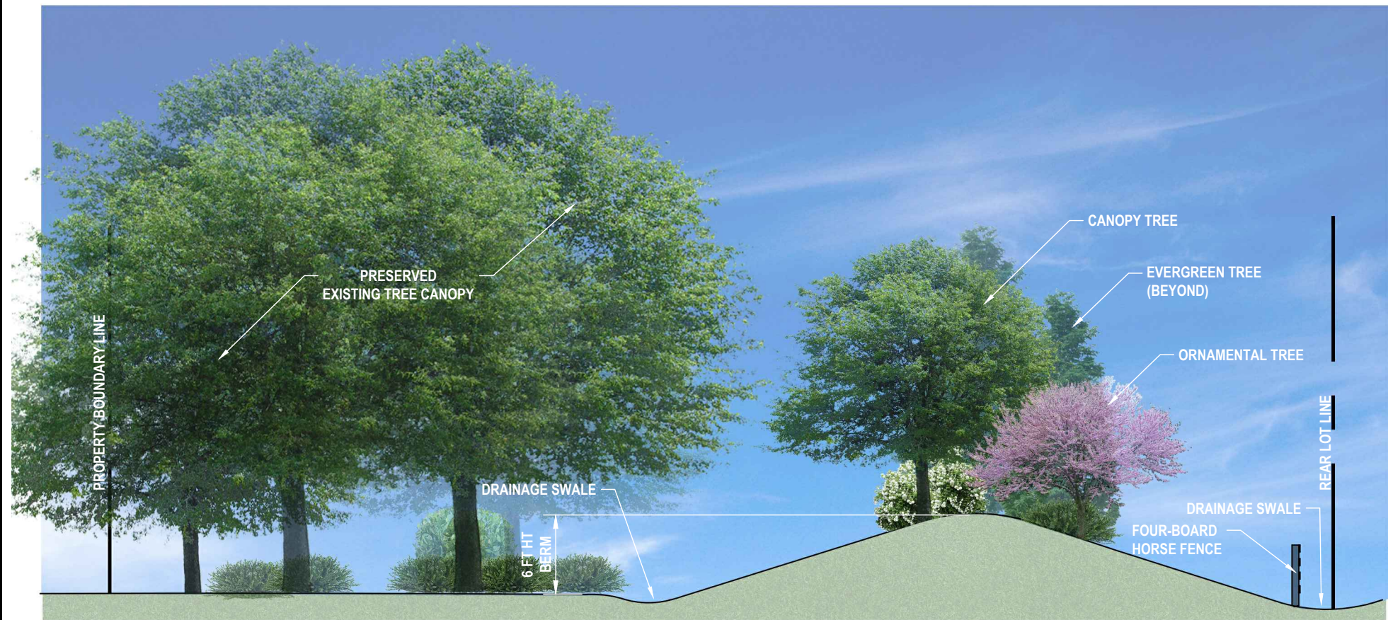
BUFFER YARD - CROSS SECTION A-A
