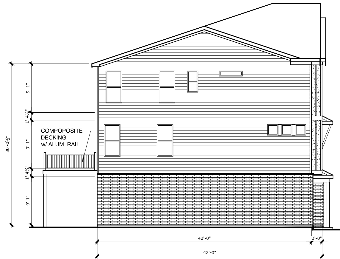
LEFT SIDE HIGH BRICK ELEVATION
