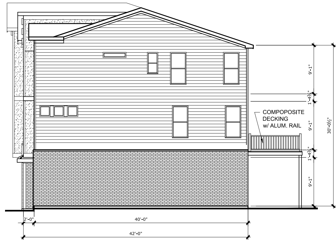
RIGHT SIDE HIGH BRICK ELEVATION
