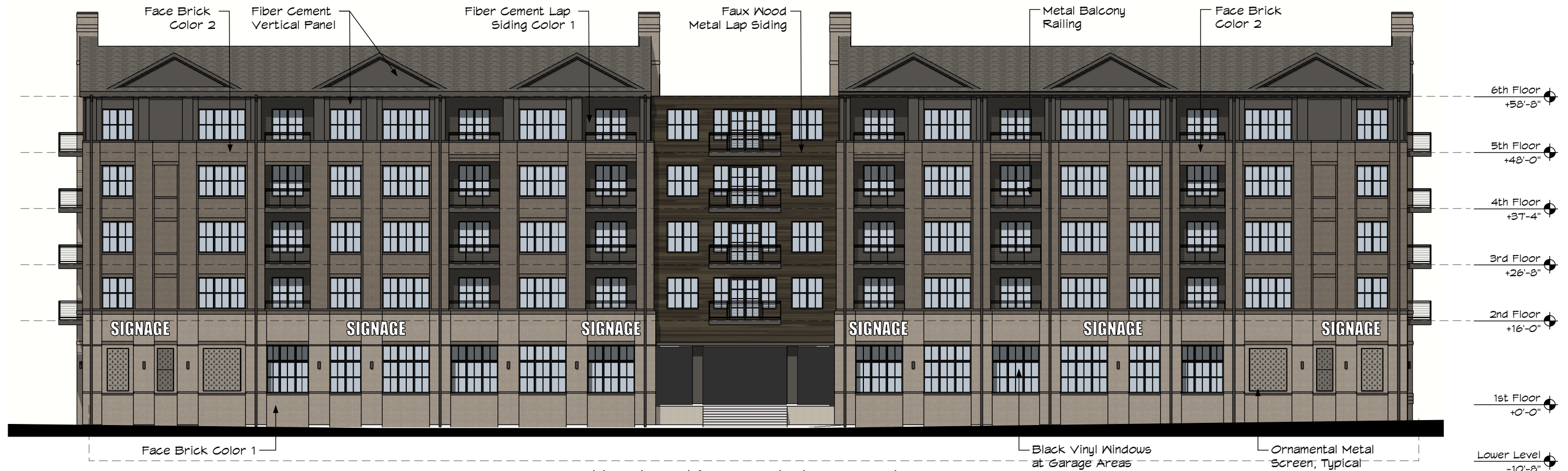
North Elevation / State Road 32
