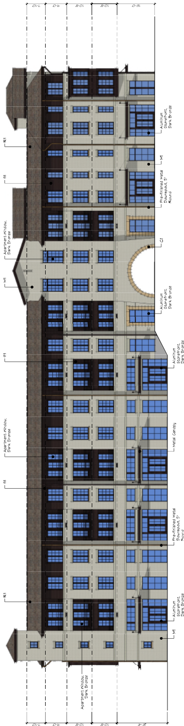
02 | BUILDING A NORTH ELEVATION SCALE 3/32" = 1'-0"
