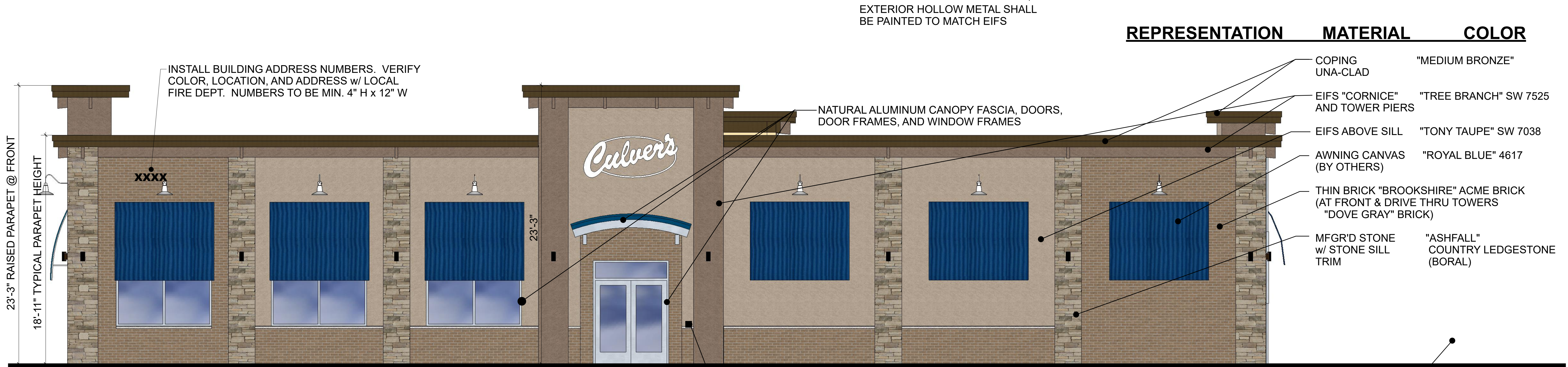
MAIN ENTRY / NORTH ELEVATION
