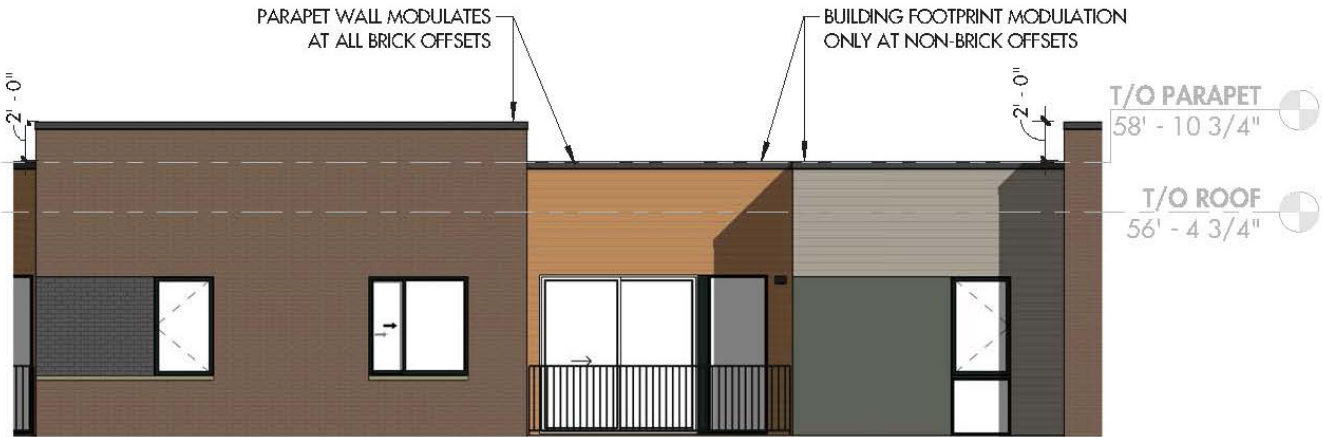
ROOF MODULATION @ BRICK OFFSETS, TYPICAL
