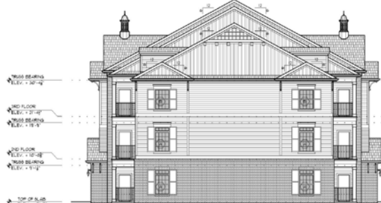
2 BUILDING TYPE II - SIDE EXTERIOR ELEVATION SCALE 1/8" = 1'-0"
