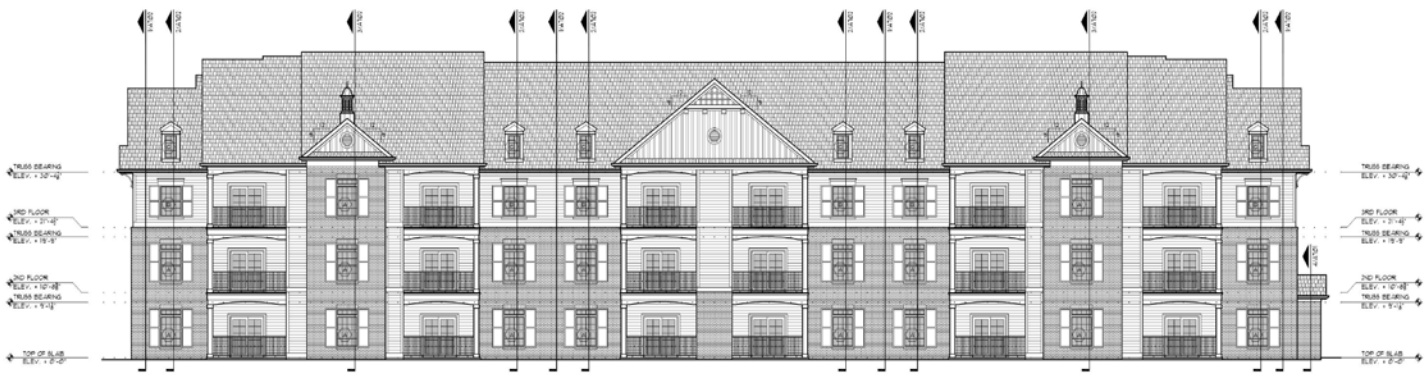
3 BUILDING TYPE I - REAR EXTERIOR ELEVATION SCALE 1/8" = 1'-0"
