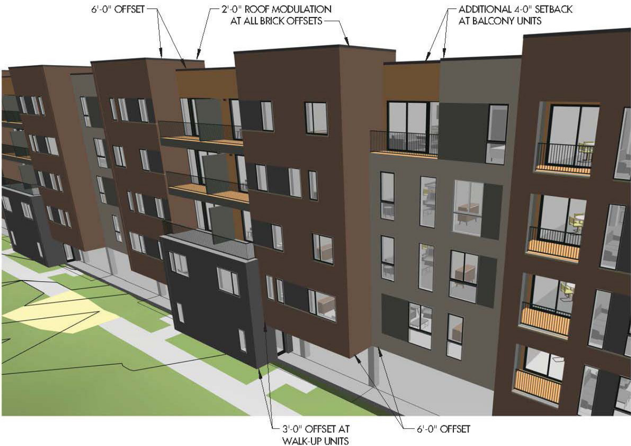
ROOF MODULATION & BUILDING OFFSET AERIAL
