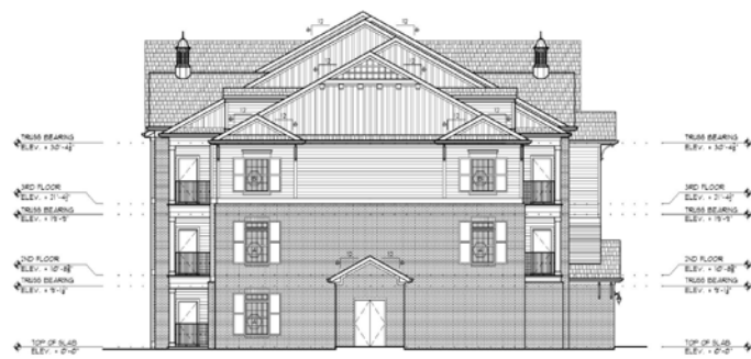
1 BUILDING TYPE I - SIDE EXTERIOR ELEVATION SCALE 1/8" = 1'-0"
