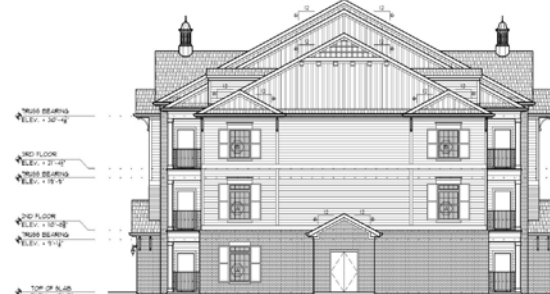
1 BUILDING TYPE II - SIDE EXTERIOR ELEVATION SCALE 1/8" = 1'-0"
