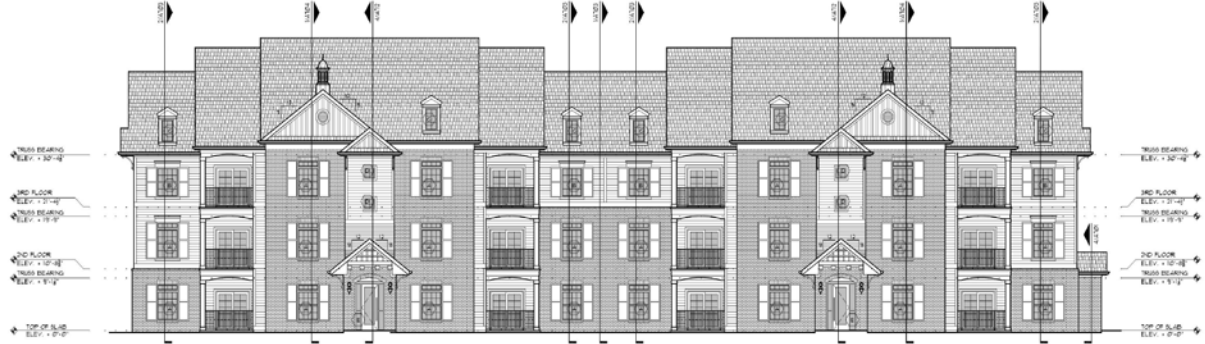
3 BUILDING TYPE II - REAR EXTERIOR ELEVATION SCALE 1/8" = 1'-0"
